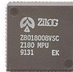
Z80180 feature-rich microcontroller running at up to 33Mhz
